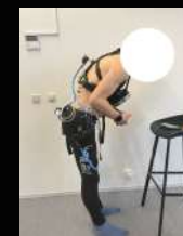
Example of a stoop-technique posture with the Laevo FLEX
